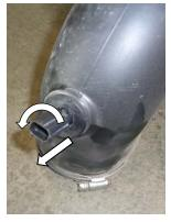
4. With the stock air intake assembly lying on a flat surface, remove the stock air temperature sensor from the intake tube by twisting counter-clockwise and gently pulling outward simultaneously. Next, remove the O-ring from the sensor body and lube the area with a sensor-safe grease. Retain in a safe place.
