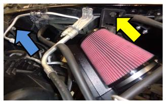
16. Reinstall the two previously removed bolts on the fender → and the front cross-frame → to secure the FM air-intake assembly. Check all fitment /fasteners and reattach the negative battery cable. Enjoy!
