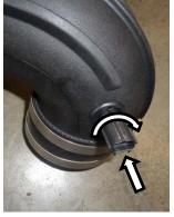
14.Install the provided rubber grommet into the hole on the FM intake tube and insert the previously retained air temperature senor fully by twisting clockwise and pressing in at the same time.
