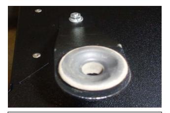
11. Next, insert the rubber grommet that was previously retained from the stock air-box into the large hole on the single-bolt bracket on the base of the heat shield so that the beveled hole faces down.
