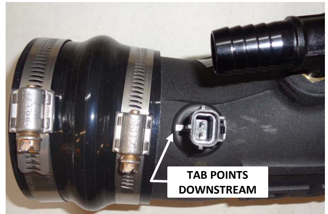
16. Carefully insert the inlet temperature sensor into the grommet, ensuring that the tab points downstream. (NOTE: Moistening the grommet with soapy water will ease insertion.)
