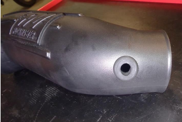
18. Insert the rubber grommet (20) into the tube. (Moistening the grommet with soapy water will ease insertion.)
