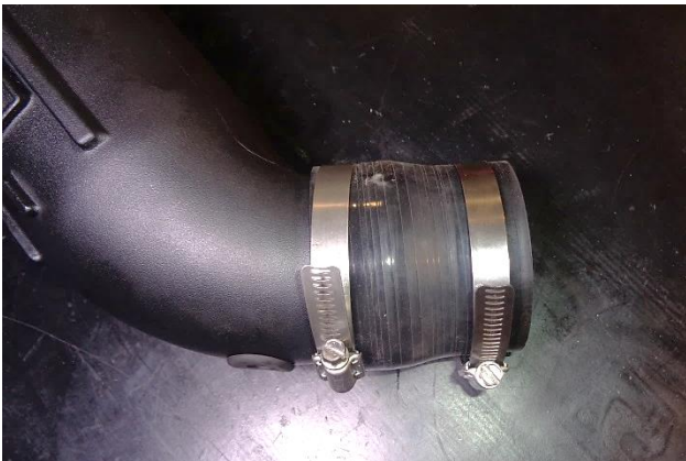
19. Slip the #52 screw clamps (24) onto the reducing coupler (25), and install the large end of the coupler on the discharge end of the intake tube. Do not tighten the clamps at this time.
