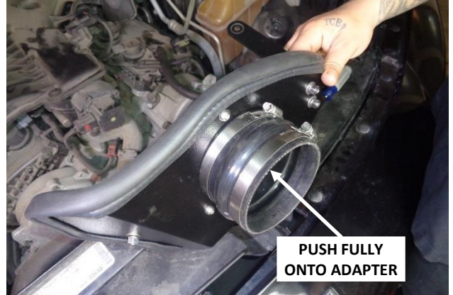
15. Slip the #56 screw clamps (17) onto the 4" coupler (18), and install the coupler on the filter adapter. Push the coupler up against the heat shield and tighten the adapter clamp.
