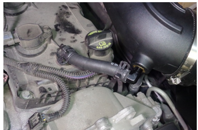
23. Cut the 1/2" hose (23) to fit between the barbed elbow and the engine's PCV fitting. Then install the hose and secure both ends with pinch clamps (22).
