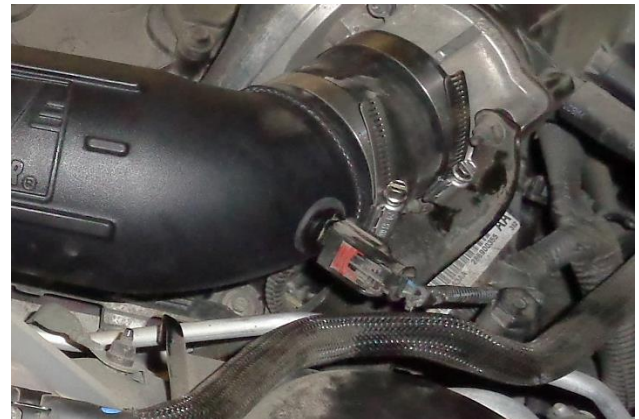
22. Connect the air temp sensor plug to the sensor, close the latch, and check the plug for security.
