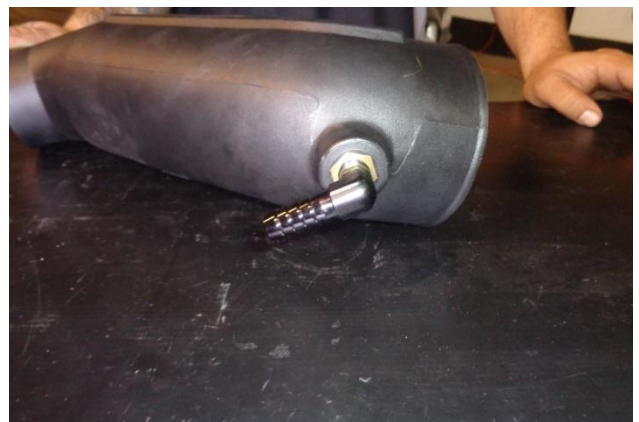
17. Apply 2 wraps of nylon thread tape to the threads of the barbed elbow (21), and install it in the intake tube (19) as shown.
