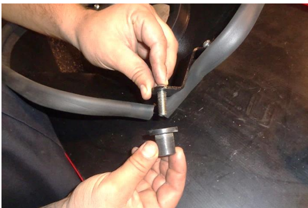
14. At bracket (5), thread the well nut (4) onto the 3/8-16 screw (6). NOTE: Hand tighten only at this time.
