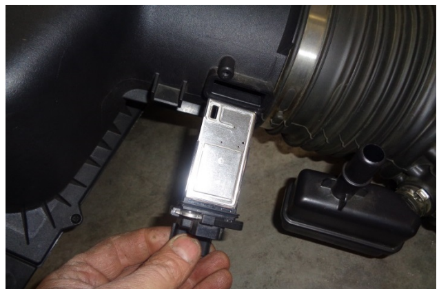
11. Remove the MAF sensor from the intake tube, then remove the stock gasket from the sensor. CAUTION: The sensor is delicate! Handle it with care, and store it in a safe location until reinstallation. NOTE: We highly recommend that you retain all factory air intake system parts.
