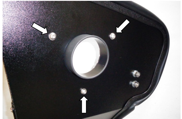
15. Attach air filter adapter (3) to airbox using M6 screws (12), lock washers (10) and flat washers (8).
