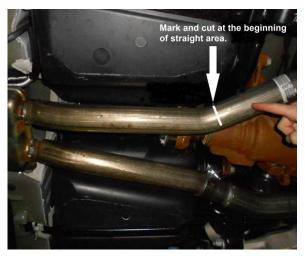
2) Begin by marking both resonator exit pipes at the beginning of the straight area as shown in the photo at left. Support the exhaust system both in front and behind the area to be cut. Check that the marks are correct, then using a sawsall, cut both pipes at the marks. Note: Due to the closeness of the pipes to the gas tank, use caution when cutting! Carefully deburr the end of the muffler inlet pipes where cut with a file or die grinder.
