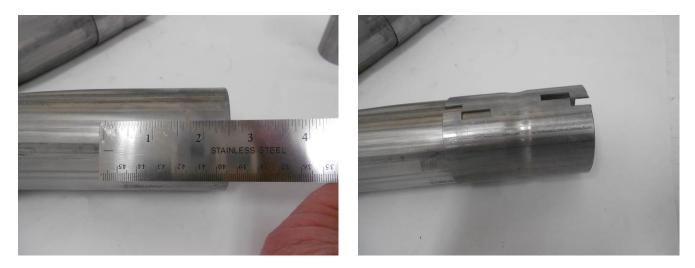
1) When using the **#86341S** X-Pipe assembly with the factory Mustang mufflers, you must first trim 2.50" from the end of both pipes at the back of the assembly. Make a mark 2.50" from the end of both pipes and cut using a hacksaw or sawsall. Use a file or die grinder to remove any burrs from the pipe ends. After cutting, slide on the **TB809S** adapter pipes onto the end of each outlet pipe. Place a supplied clamp onto the connections and tighten enough to hold.
