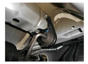
3) Using a 13mm wrench, loosen the two hangers just behind the rear differential from the cross member and the two hanger mounts at the rear of the vehicle from the frame. Slide the muffler assemblies toward the rear of the vehicle to disengage them from the factory system. Leave them hanging in place for re-assembly onto the Flowmaster X-pipe assembly.
