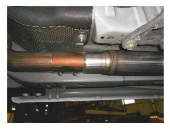
2) Be sure that the factory band clamp from the resonator inlet is in place on the front pipe behind the catalytic converters. Place the Y-pipe assembly **#86320S** up into position behind the factory front pipe and slide into the clamp until it stops. Support the rear of the Y-pipe with a stand and tighten the clamp enough to hold, but still allow for adjustment. The Y-pipe outlet with two bends will be oriented to the drivers' side of the vehicle.
