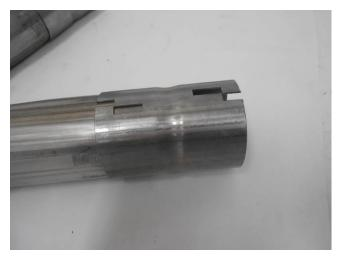
1) Slide a supplied **TB810S** adapter pipe onto the end of each outlet of the **86320S** Y-pipe assembly. Place a supplied clamp onto the connections and tighten enough to hold.
