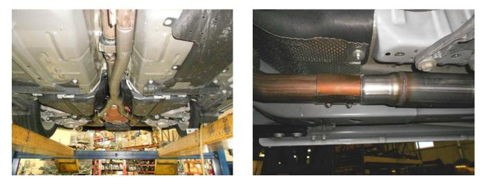
1) Be sure that the factory band clamp from the resonator inlet is in place on the front pipe behind the catalytic converters. Place the Y-pipe assembly **#86320S** up into position behind the factory front pipe and slide into the clamp until it stops. Support the rear of the Y-pipe with a stand and tighten the clamp enough to hold, but still allow for adjustment. The Y-pipe outlet with two bends will be oriented to the drivers' side of the vehicle.
