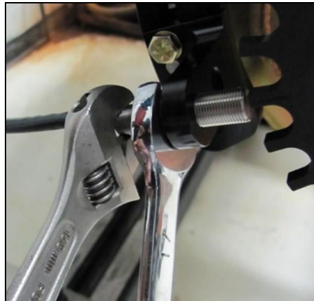
Figure 9: Locking the sensor gap.
