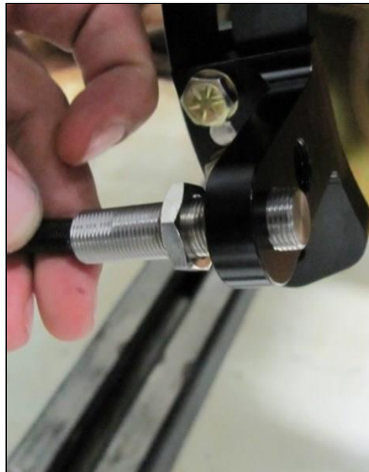
Figure 3: Installing the sensor.
