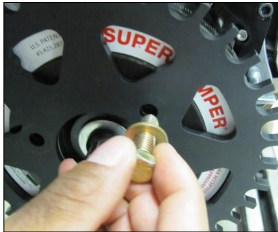
Figure 7: Fastening the crank wheel to the balancer.
