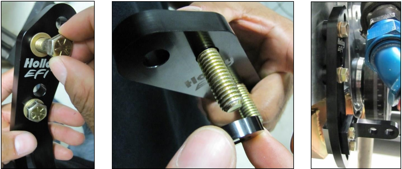
Figure 4: Mounting the engine-block bracket to the engine.
