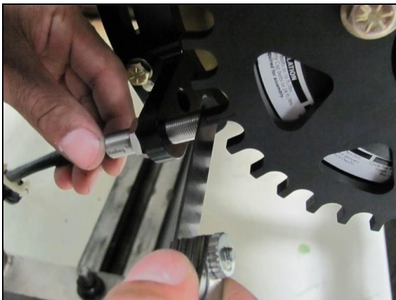
Figure 8: Adjusting the sensor gap.
