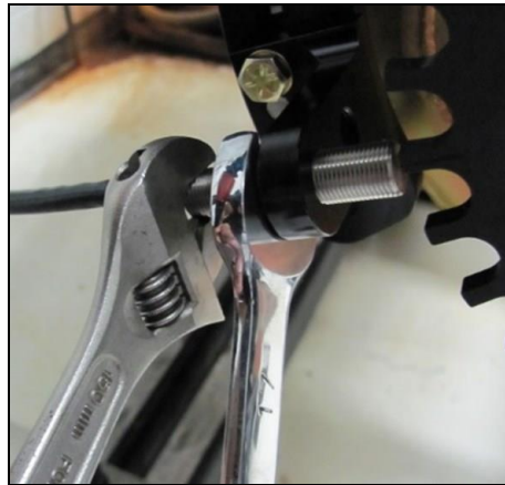
Figure 4: Locking the sensor gap.
