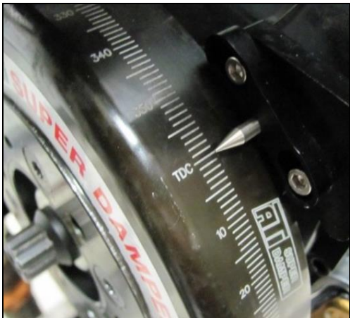
Figure 1: Rotating the engine to TDC #1.
