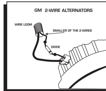
Figure 5 Installing the Diode to a 1973-1983 GM Vehicle.
