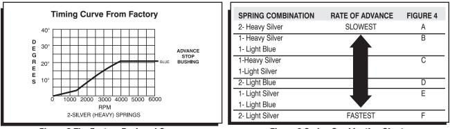
Figure 2 The Factory Equipped Curve.
