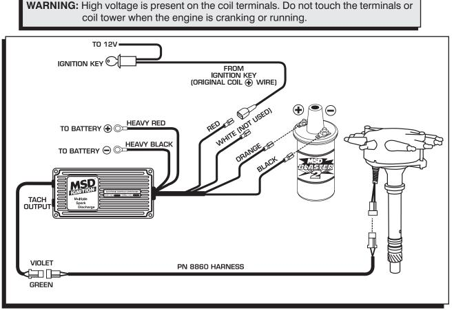
Figure 10 Wiring to an MSD 6-Series Ignition Control.
