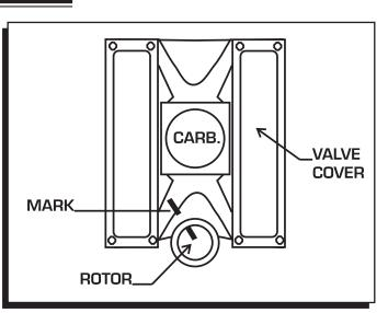
Figure 8 Marking the Rotor Location.
